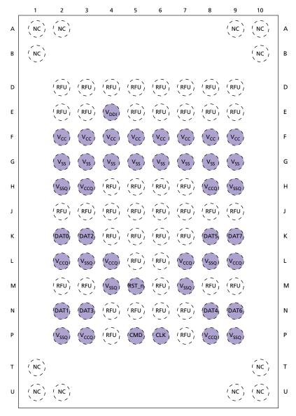
Note: 1. Connect a  $1\mu F$  decoupling capacitor from  $V_{DDI}$  to ground.
