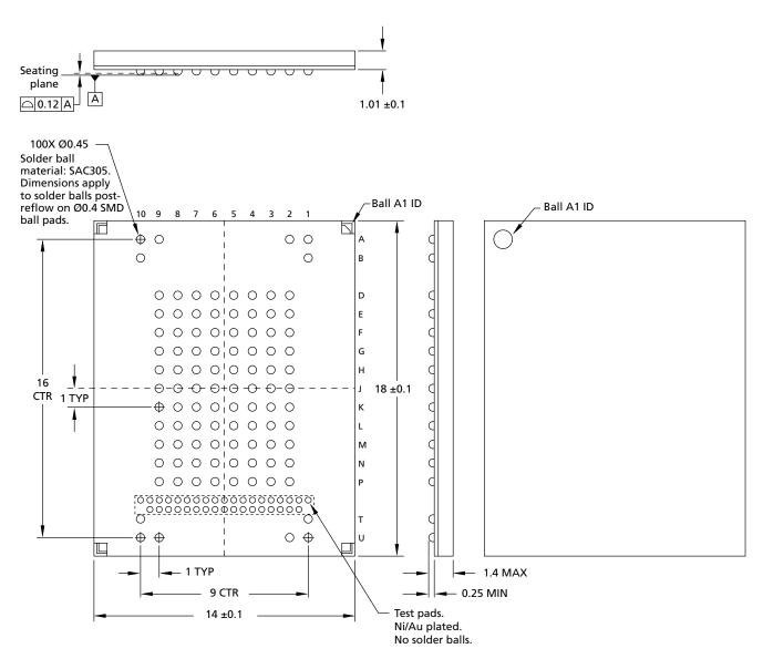
Note: 1. Dimensions are in millimeters.
